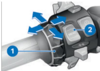
The navigation system is operated using the Multi-Controller **1** and the rocker button **MENU 2**.
