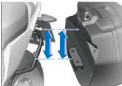
If a case wobbles or is difficult to fit, it must be adapted to the gap between the upper and lower mount.
