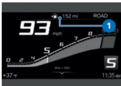
The range **1** indicates how far you can ride with the remaining fuel. This distance is calculated based on average consumption and the remaining fuel quantity.
