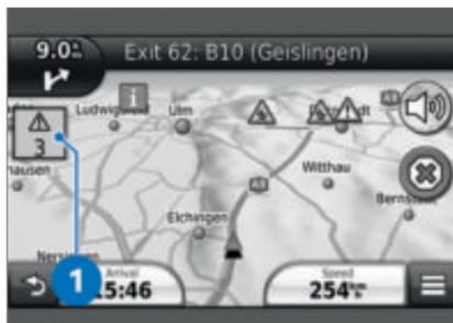
Warning and status displays of the motorcycle are indicated with a corresponding symbol **1** at the upper left on the map view.
