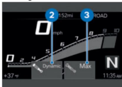
The new chassis and suspension adjustment options for damping **2** and spring setting **3** are displayed for a short period of time.
