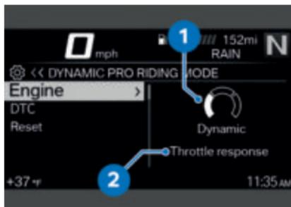
The Engine system is selected. The current setting is displayed as a diagram 1 with explanations of the system 2.
