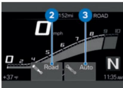
Immediately after the button **1** is pressed, the chassis and suspension adjustments options for damping **2** and spring setting **3** are displayed.
