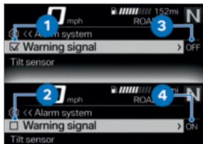
Some items are preceded by a box. The box indicates whether the function is turned on or switched off. Action icons after the menu items illustrate what is switched by briefly tilting the Multi-Controller to the right.
