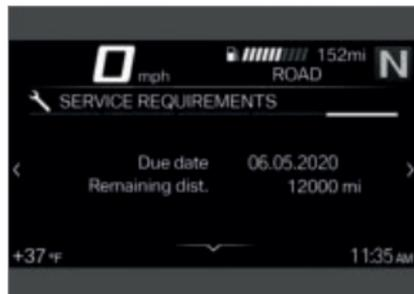
If the time remaining until the next service is less than a month, or if the next service is due within 700 mi (1127 km), a white **Check Control** message is displayed.
