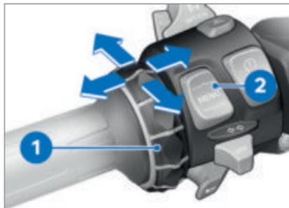
All contents of the display are controlled by the Multi-Controller **1** and the rocker button MENU **2**.
