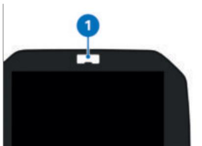
The shiftpoint light **1** signals to the rider that the engine speed is approaching the RPM at which the rider needs to shift to the next highest gear.
