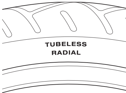
Typical Tire Marking - Tubeless Tire
